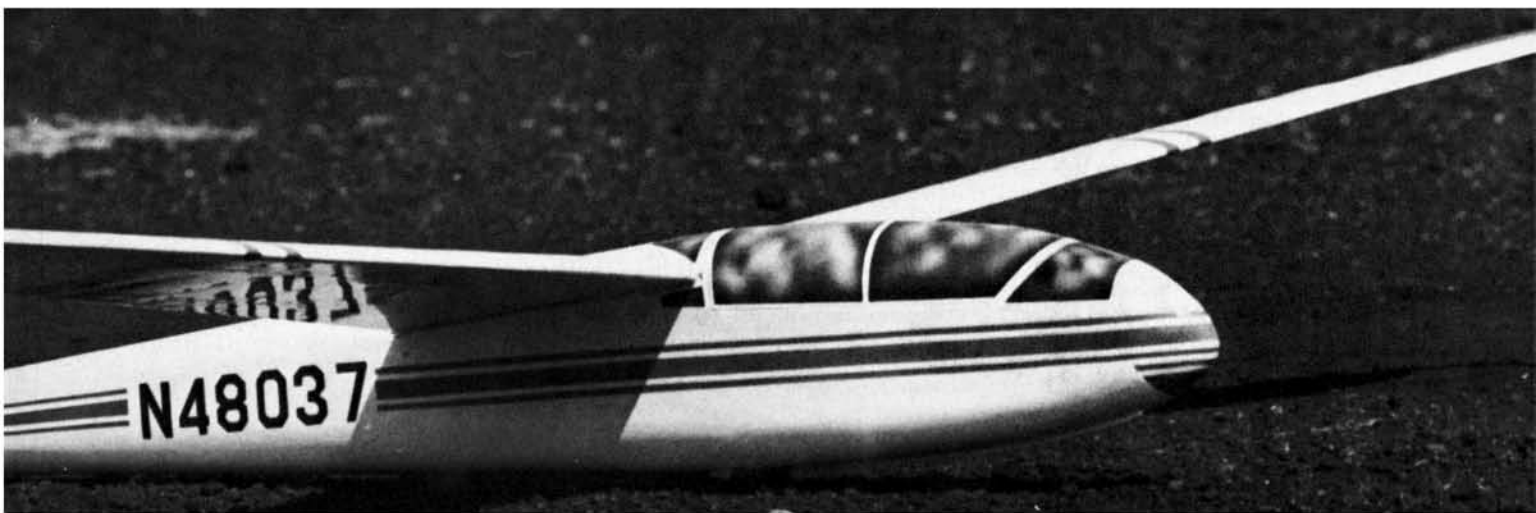
Long Island Soaring Association's Blanik L-13 touches down at Brookhaven Airport. Notice dive brakes/spoilers extended. Facing page: Bob's model replica. Wing is swept forward a few degrees, visible when overhead. Below: A like-angle on model Dihedral increased 2 degrees, canopy simulated. It spans 72".
